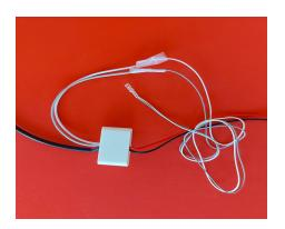
1. Connect the white and grey wires from receptacle to LED. White wire from receptacle is POSITIVE. Grey wire from receptacle is NEGATIVE. Wrap exposed wires with tape.
