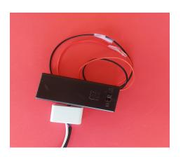
2. Connect red and black wires from receptacle with battery box (red with red; black with black). Wraps exposed wires with tape.
