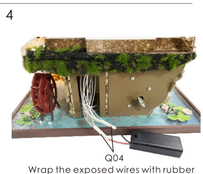
Wrap the exposed wires with rubber
