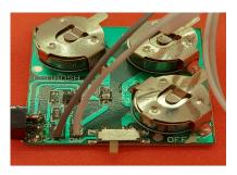
3. Insert 3x LR44 batteries (INCLUDED) into the slots and toggle the white switch to ON.
