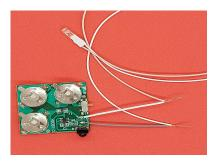
1. Connect LED with receptacle (white with grey). White wire on receptacle is POSITIVE; Grey wire on receptacle is NEGATIVE.
