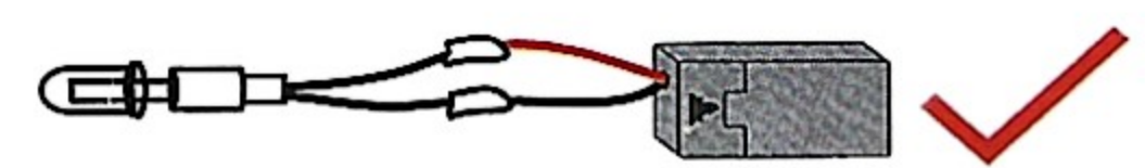
Use batteries with the box to test the light can work or not!
